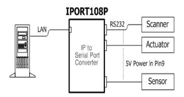
This is one structure for test equipment used in iPhone's production line. And you can have similar structure in your next application environment. IPORT108P box is your solution.
