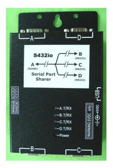
★ Any data from master port A will be sent to slave port B, C, D simultaneously.
