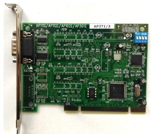
★ Port interface can set to target RS232/RS422/RS485
