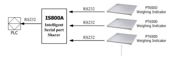
In this condition any device without ID code to differentiate can use IS800A to let multiple devices to work with PLC. If there were ID code in device to differentiate device, then we can use standard IS800 box to work with PLC. In IS800 box we will not modify any data from slave port to PLC. In IS800A box we will add ID code in data from slave to PLC.
