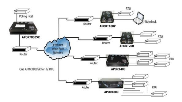
If your application environment might ask one host to connect more than 32 RTU devices, then we may need to add one S272 serial port sharer between host RS232 serial port and each APORT800SR box. The master port of S272 box will connect to host RS232 port. The slave port of S272 box will connect to APORT800SR box. Because we have 7 slave ports in one S272 box, so we can connect up to 32\*7=224 RTU devices in application environment as following figure.
