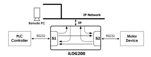
In this condition we can check the command from operator and the status response from machine. When there is abnormal function in machine, we can check the command from operator and status response from machine. Then it is very easy to find the possible reason for such abnormal condition.
